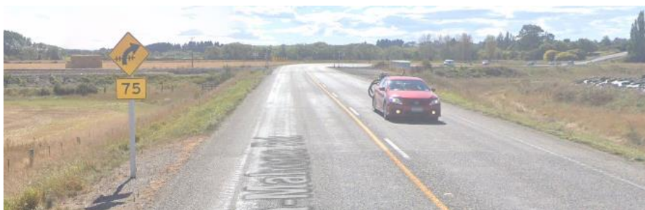
Figure 6-4: Curve/rail line sign upstream of the Alma Mahino Rd crossing prior to a curve
